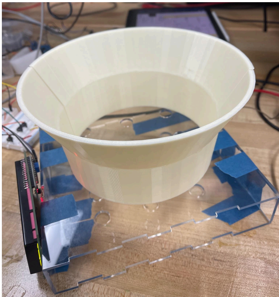
Figure 29. The laser cut box, above which lies the outer encapsulation of the physical subunit. It is turned upside down to accommodate the large radius of the spinning tubes.
