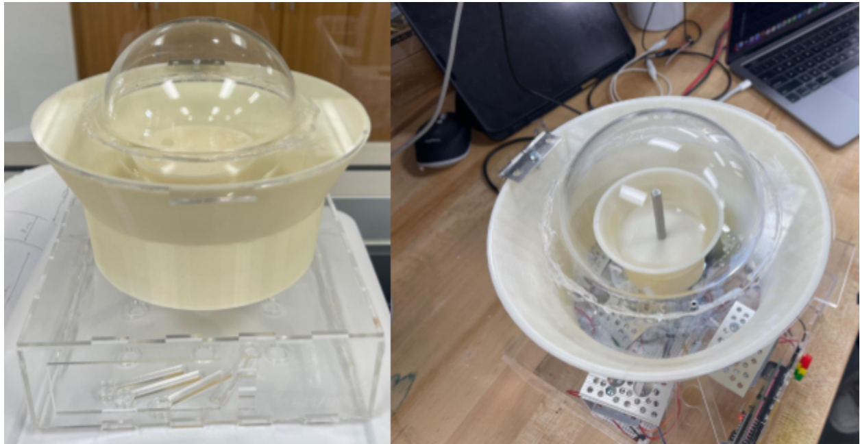
Figure 42. Our next step in V3 integration was attaching the laser-cut lid to the preordered dome. On the left is a front facing picture of the system and on the right is a top-down picture that highlights the hinge and motor inside.
