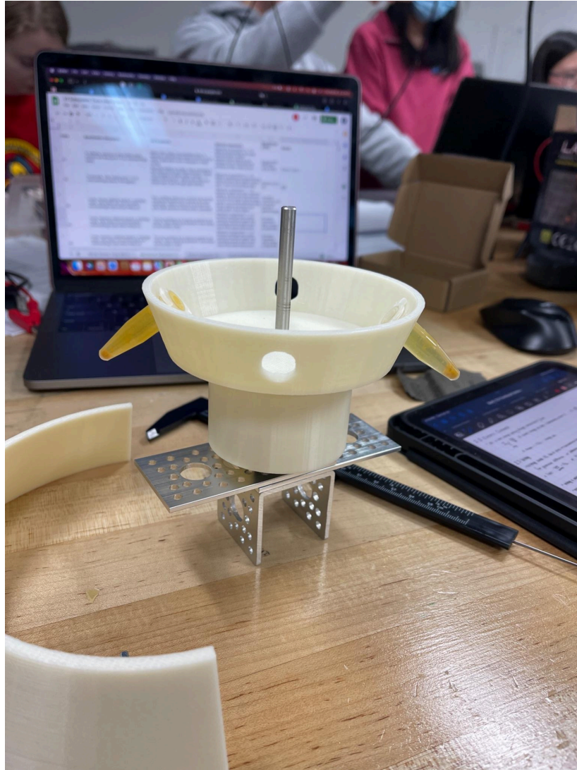
Figure 25. The internal physical complex resting on a base designed from M6 components. The motor is housed inside the shown unit.
