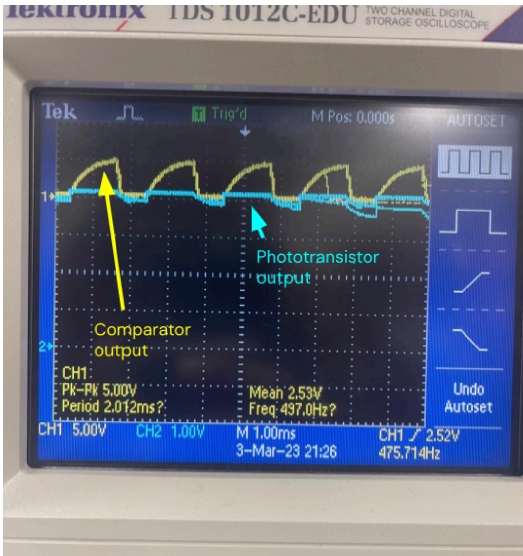
Figure 51. An oscilloscope readout showing the voltage differences in both the comparator and the phototransistor. The matched rise in both indicates that the comparator is successfully interpreting a change in light that the phototransistor receives.
