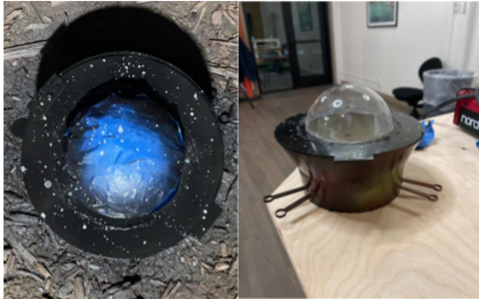
Figure 49. The V3 external encapsulation during (left) and after (right) its spraypainting. Blue tape was used to cover the domed region so that it remained clear even after being painted.
