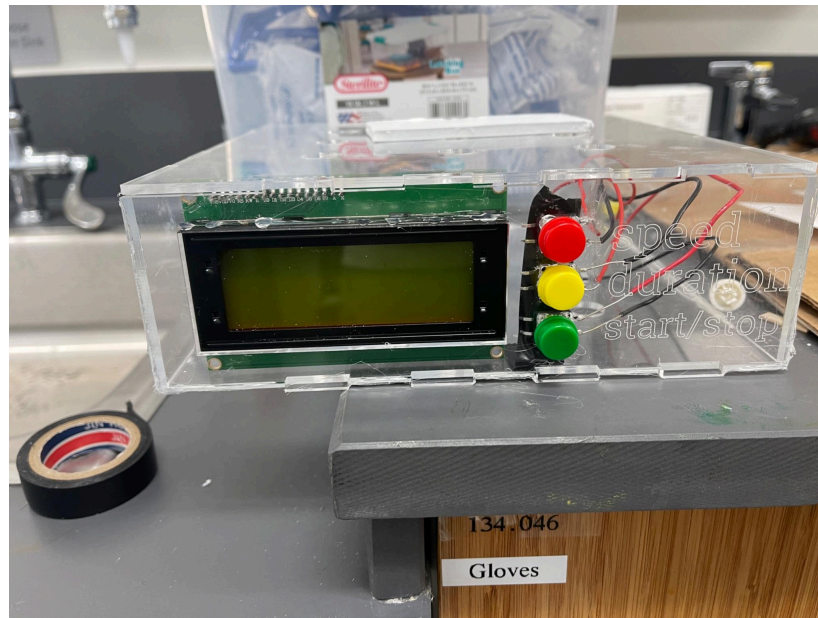
Figure 43. The next big step in V3 integration, where the buttons and LCD screen were placed into the front face slots.
