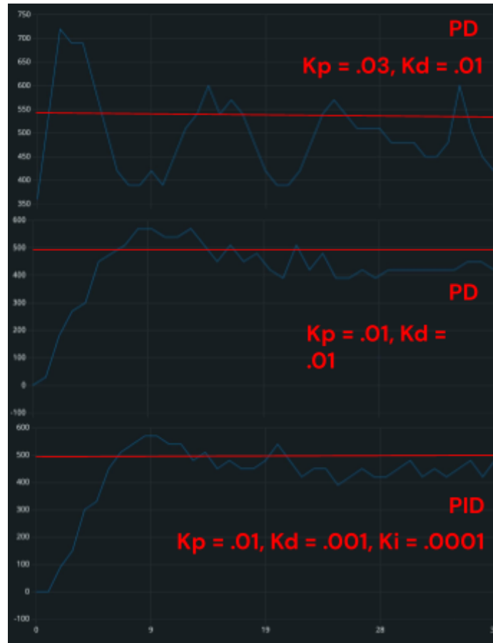
Figure 10. shows iterations of our control system software through three different time (seconds) vs RPM graphs with a goal RPM of 500. From top to bottom, the control system becomes more accurate both in time to stabilization and stability. The first two iterations were PD control systems and the last has integration incorporated. We left V3 using the
