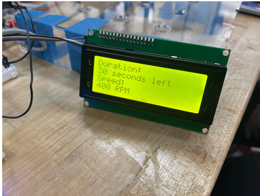
Figure 34: The LCD display and the messages it displays while the motor is running. Seconds count down until 0, at which point the motor stops. The speed is supposed to be displayed live through the phototransistor complex, but never functioned appropriately throughout the build.
