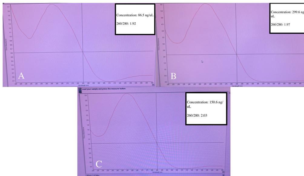
*Figure 5: Results of testing three strains of pET-21\_GH109-GFP via Nanodrop spectrophotometry. Figure 5A corresponds to the subcloning strain, 5B corresponds to the high efficiency strain, and 5C corresponds to the BL21 strain. Graph is plotting absorbance vs wavelength (nm). Tests also indicated both concentration and the 260/280 ratio, listed on the right of each figure.*
